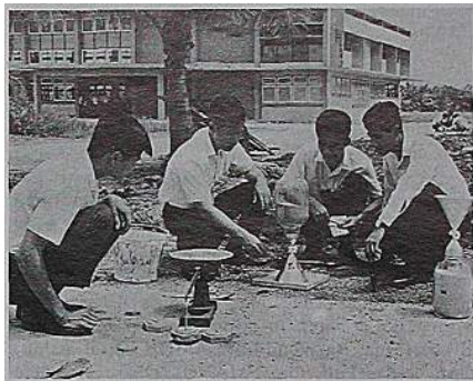
The Thonburi Technical Institute, in Bangkok, was established in 1960 to train technicians and engineers in order to supply the growing industries with the necessary technical personnel. The United Nations Special Fund is assisting the Institute with UNESCO serving as Executing Agency. Students learning Soil Volumetry by sand method. In the background is the Foundry Shop. (United Nations).
