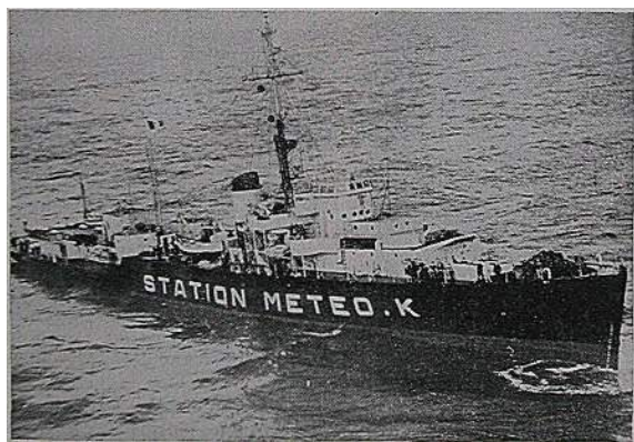
Ocean Weather Station. Weather ships in various oceans make regular weather observations at positions fixed by international agreement to provide continuous data from points essential for air navigation. Shown here is French weather ship K in North Atlantic. (WMO photo)
