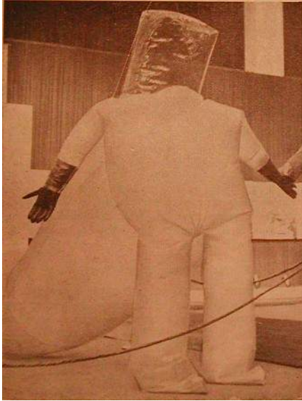
"The Human Dragon". This protective suit, with a tail much longer than a man is tall, is worn by United States workers who crawl into the suit through the tunnel-like tail. It protects them from radioactive dusts and gases. The ILO has been fighting dust diseases and explosions for many years.
