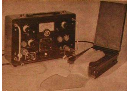
Fig. 4. Gloves monitor for checking radioactive contamination.
